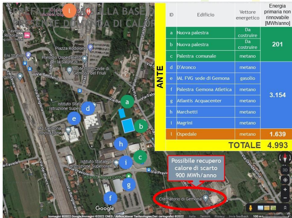
Figure 2: buildings to be connected at various project implementation stage and non-renewable primary energy
